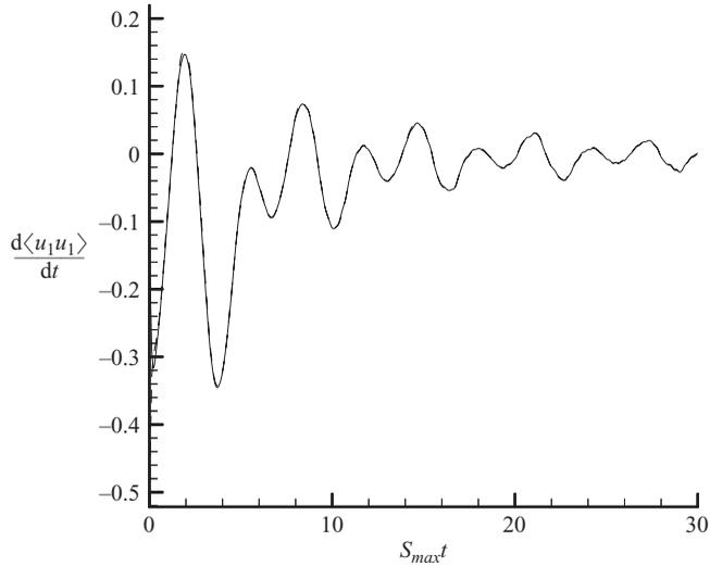
FIGURE 20. Comparison of  $d\langle u_1 u_1 \rangle / dt$  computed from —, numerical differentiation of  $\langle u_1 u_1 \rangle$  and ---, the right-hand side of (3.24) in the  $\omega/S_{max} = 1.0$  case.  $\langle u_1 u_1 \rangle$  is normalized by  $\langle u_1 u_1 \rangle$  at  $t = 0$ .
