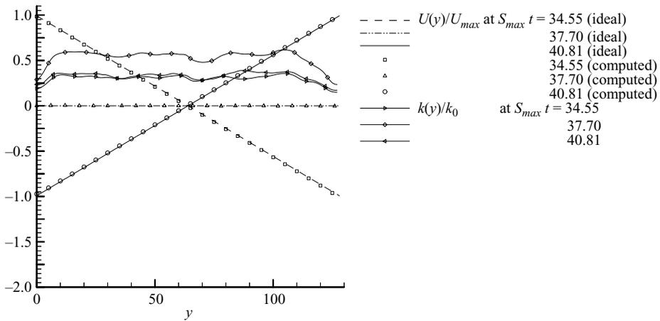
FIGURE 5. The profiles of  $U(y)$  and  $k(y)$  at  $S_{max}t = 34.55, 37.70$ , and  $40.81$  for  $\omega/S_{max} = 0.5$ . Ideal vs. computed.
