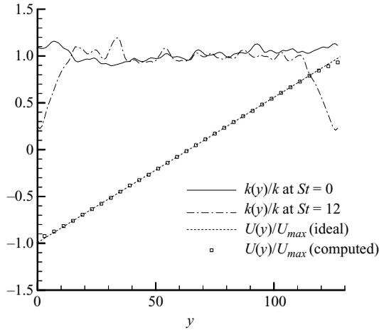
FIGURE 2. The profile of mean velocity at  $St = 12$  and the distribution of  $k(y)$  at the initial stage and  $St = 12$ . The wall effects are limited to regions near the walls. In the inner region, mean velocity agrees well with the ideal mean velocity and homogeneity of turbulence is maintained.
