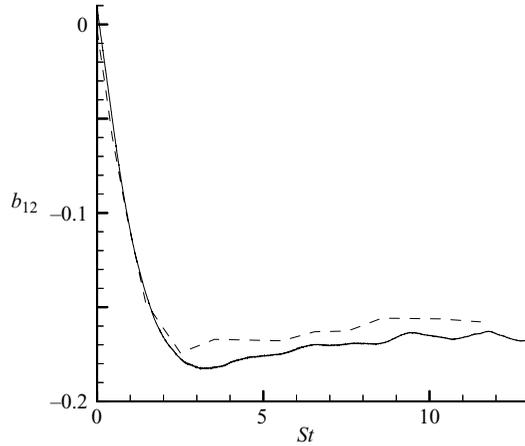
FIGURE 4. The results of  $b_{12}$  obtained from —, DNS using LBM and ---, Navier–Stokes equations by Jacobitz, Sarkar & Van Atta (1997) with initial values of  $Re_\lambda = 44.72$  and  $Sk/\varepsilon = 2.0$ .
