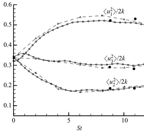
FIGURE 3.  $\square$  Evolution of normal Reynolds stress in homogeneous turbulent shear flow (constant shear).  $\triangle$  NS-DNS data are from Rogers (1986) with initial values of  $Re_\lambda \approx 35$  and  $S^* = 1.2$ .  $\bullet$ , Experimental data are from Tavoularis & Corrsin (1981a) with  $Re_\lambda = 284$  at  $St = 8.6$ .
