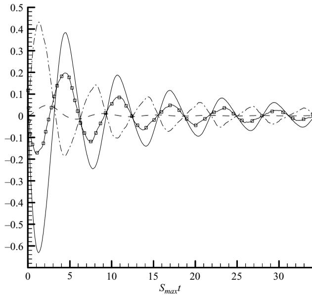
FIGURE 21. Temporal variation of the  $\langle u_1 u_2 \rangle$  budget in the  $\omega/S_{max} = 1.0$  case. —, production; ---, dissipation; -·-, pressure redistribution; -□-,  $d\langle v_1 v_2 \rangle / dt$ . All terms are normalized by  $\langle u_1 u_1 \rangle$  at  $t = 0$ .
