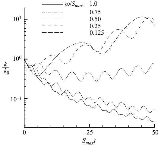
FIGURE 9. Evolution of  $k$  in various  $\omega/S_{max}$  cases.
