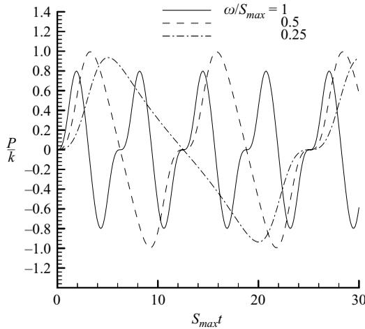
FIGURE 28. RDT production of  $k$  for  $\omega/S_{max} = 0.25, 0.5$  and  $1.0$ .
