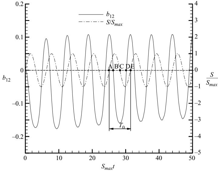
FIGURE 15. Evolution of  $b_{12}$  in the  $\omega/S_{max} = 1.0$  case.
